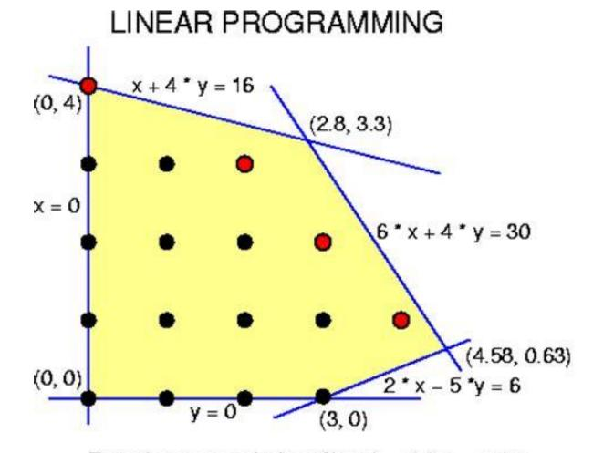
Function to maximize: f(x, y) = 6 \* x + 5 \* yOptimum LP solution (x, y) = (2.4, 3.4)Pareto optima: (0, 4), (2, 3), (3, 2), (4, 1)Optimum ILP solution (x, y) = (4, 1)
